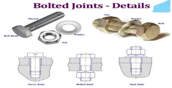
Components of a Bolted Joints 1. Bolt 2. Washer 3. (and/or) Nut . Different combinations of the above may be used for a joint depending on the load.12.9 Class Bolt/Nut Means 12.9
