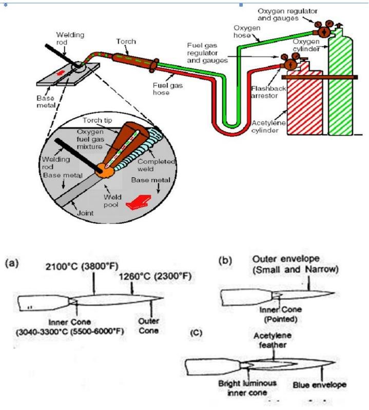
The first reaction takes place when the fuel gas such as acetylene and oxygen mixture burns releasing intense heat.
